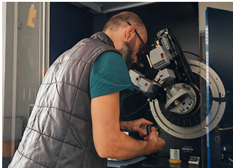
FIG. 13 Inserting a sample holder into an X-ray powder diffractometer Bruker D-8 DISCOVER. Photo by R. Skála.
