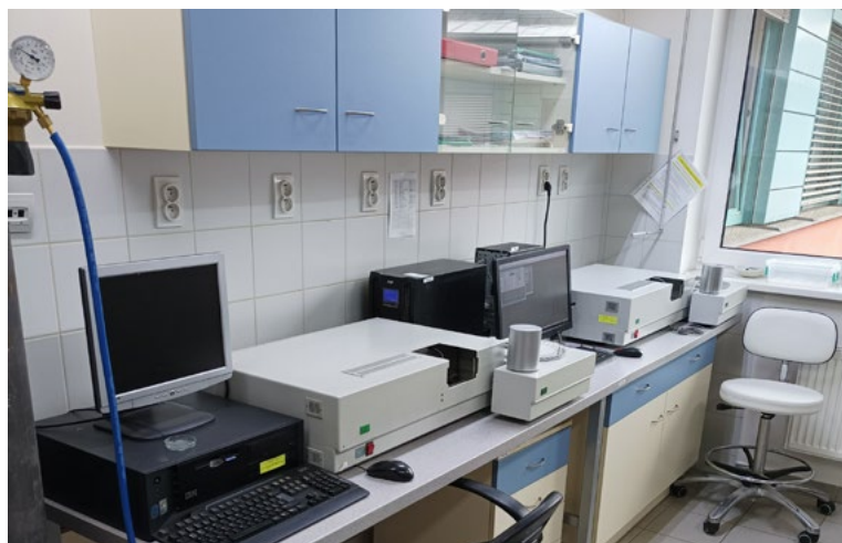
FIG. 14 A pair of cold vapor atomic absorption spectrometers AMA-254 by Altec, Prague with autosamplers and power backup station. Photo by T. Navrátil.
