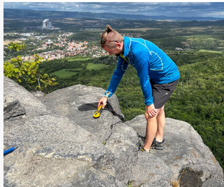
FIG. 36 Magnetic susceptibility measurement using a portable instrument to determine parameters of rocks possibly affected by lightning at the top of Bořeň Hill. Photo by H. Ucar.
