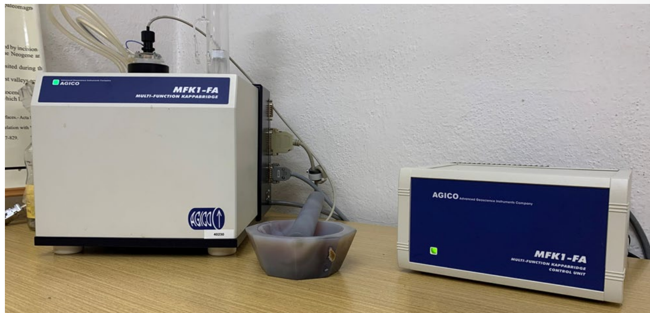
FIG. 9 AGICO MFK1-FA highly sensitive kappabridge for measuring anisotropy of magnetic susceptibility and susceptibility in variable magnetic fields, frequencies and temperatures. Photo by L. Kouklíková.
