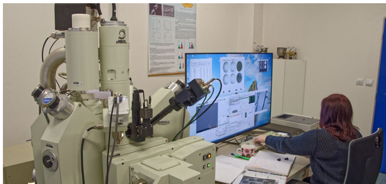
FIG. 6 Quantitative chemical analysis by an electron microprobe JEOL. Photo by R. Skála.
