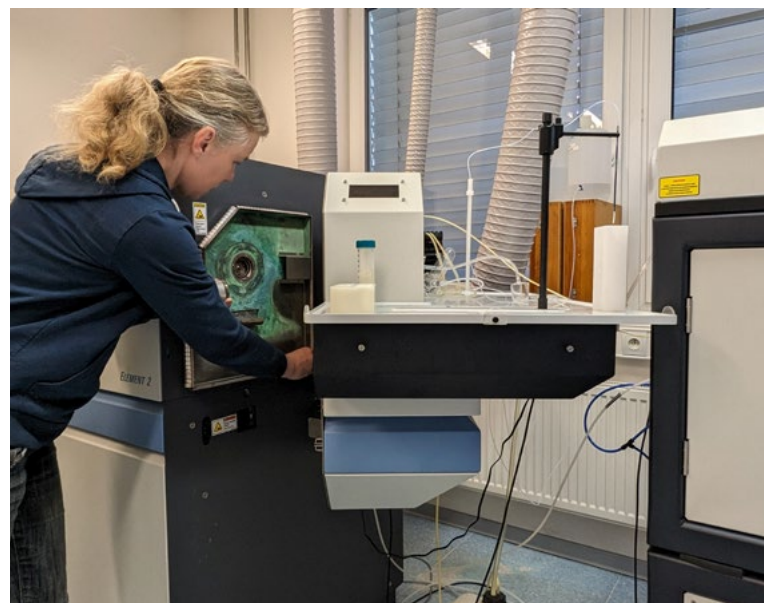
FIG. 5 Maintenance of high-resolution Element 2 magnetic sector field ICP-MS (left) connected with an Analyte/Excite excimer 193 nm laser ablation system (right) in the ICP-MS lab. Photo by M. Svojtka.
