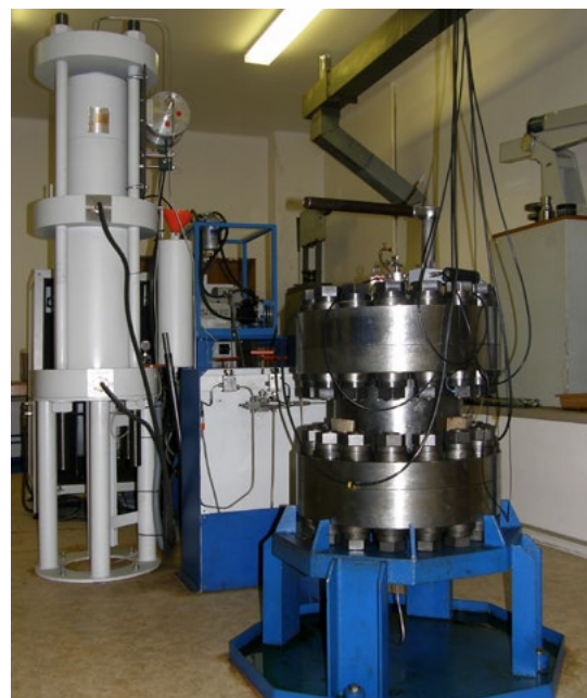
FIG. 10 Hydrostatic pressure vessel for measurement of detail, P and S wave, velocity anisotropy. Photo by V. Filler.
