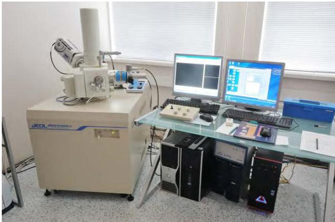
Scanning electron microscope with EDS system
