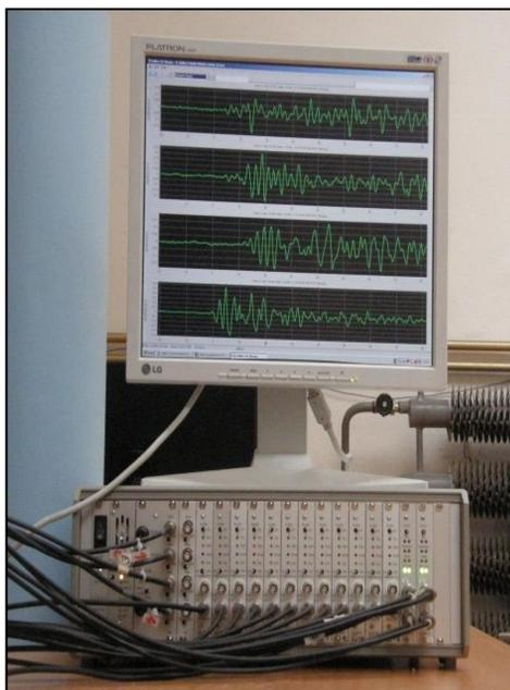
**Vallen System AMSY-5** is a sixteen-channel transient recorder which allows us to monitor process of cracking during the uniaxial loading of rock sample. A net of 16 sensors detects every single crack in rock above the limit set. Recorded data are used to localize each crack and map the process of their propagation in time. This helps us to understand better the behavior of the rock failure process.
