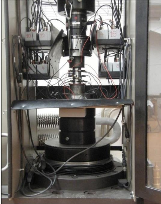
**Uniaxial load frame MTS** is a computer-controlled servo-hydraulic loading system specifically adjusted for long-term testing. This system allows testing of rocks in regime of controlled force or controlled deformation. Together with triaxial cell, this equipment allows simulation of pressure-temperature conditions and permeability measurements.
