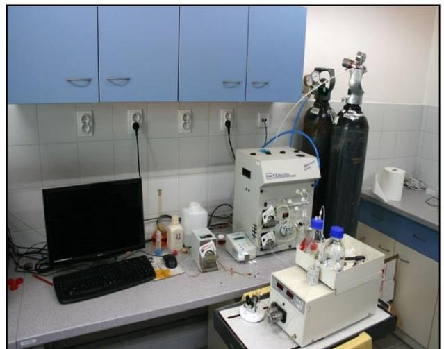
The instrument is designed for mercury analyzes in liquid samples and for speciation studies.
