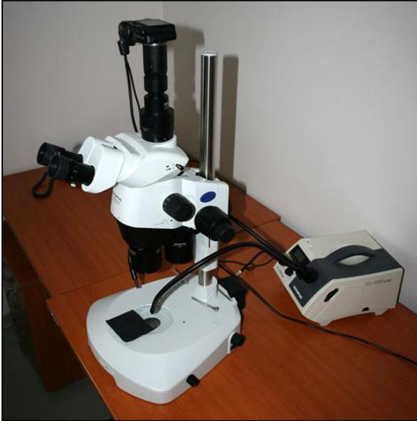
**OLYMPUS SZX 16** Optical binocular microscope with the **CANON** digital photocamera and specialized **QuickPHOTO Micro** software and a **Deep Focus module** is used for the documentation of samples, separation of sub-samples for other methods and, of course, for imaging of samples and details for publications.
