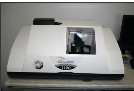
← The **CILAS 1190 LD laser granulometer** is used to provide a measurement of the grain size distribution in range from 0.04 to 2,500 μm. The measurement is based on a small amount of material and might be easily repeated. Using the different types of dispersion allows to get the picture about the primary or secondary given grain size distribution. Data can be reported in different fractions set by the user.
