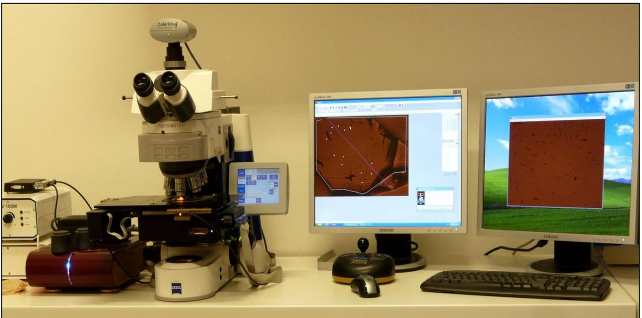
**ZEISS Imager. M1m Microscope** connected to two monitors of a computer for a fission track analysis (FTA).
