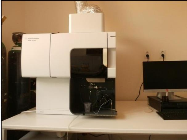
Chemical composition of samples is studied on universal multielement spectrometers in an argon plasma discharge (**ICP EOS instrument**). At temperatures about 10,000 K, chemical elements present in the sample emit visible or UV radiation, which is collected and processed. As a result, certain element is identified together with its content in the sample.
